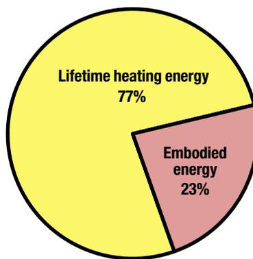
Operating versus embodied energy consumption for a typical 1970s North American wood-frame home and for a similar home designed to R-2000 standards, a Canadian program for energy efficiency. The climate is Ottawa and the life span is 30 years. This data was calculated using the HOT2000™ energy simulation software and the ATHENA™ Environmental Impact Estimator (5). In a milder climate, the embodied energy portion would be even larger.
