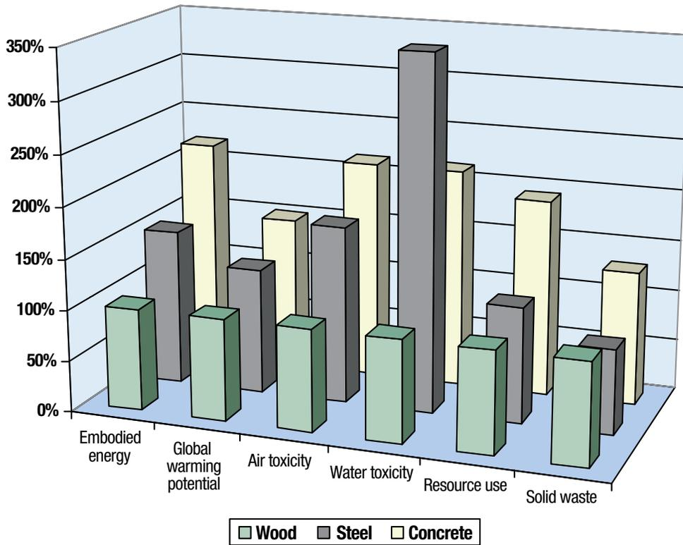
Environmental impact relative to a typical wood-frame home (the 100% baseline) is shown for an equivalent house in light-gauge steel and an equivalent in insulated concrete forms (4). Data addresses the life-cycle portion from resource extraction through construction and does not include environmental impacts of building occupancy and demolition.
